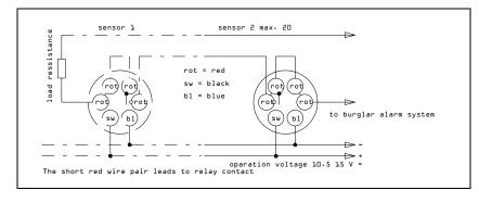
One or up to 20 **GBD** detectors can be wired in series according to the connection diagram including a termination resistor (4.7 – 22K Ohm). The wires of red and white are the relay output wires, the wires of yellow and brown are anti-tamper loop
